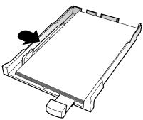
Slide the Length Guide in to fit the bottom edge of the paper.
